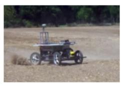
combine data-driven model(Bayesian neural network) with model-based control(model predictive control) to achieve stable path following tasks, even if the amount of data is not enough to recover the robot model. Results aims at adapting an off-road mobile robot behaviour to the diversity of encountered situations in an agricultural context. The proposed trainee will take part of experiments conducted on different robot available at INRAE.
